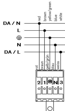
Depending on whether 3-pole, fig. left or 5-pole cables, fig. right, were used.
